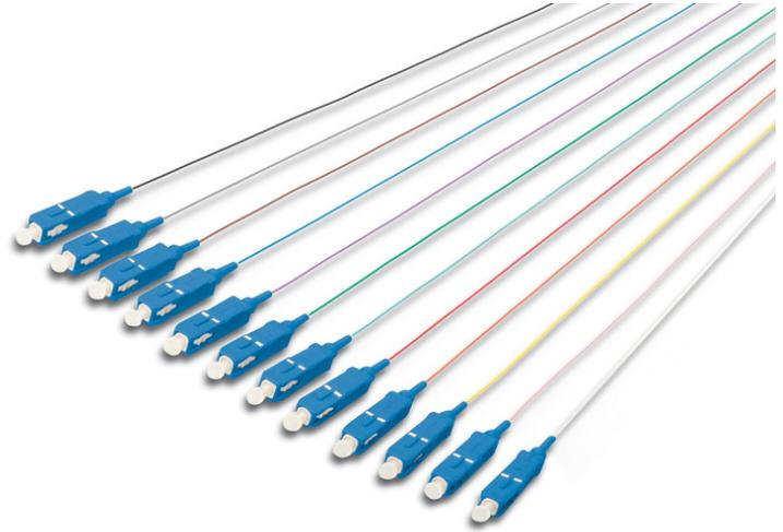
**FO pigtail set, 12 pcs., SC, SM OS2 09/125 æ loose buffer, color code DIN IEC 304, 2 m**
