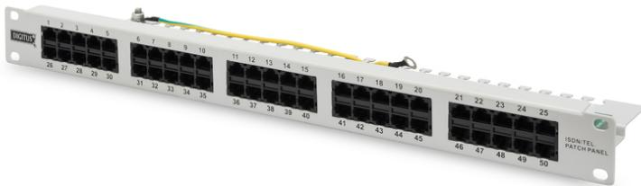
**CAT 3 ISDN Patch Panel, ungeschirmt, 50-Port RJ45, 8P4C, LSA, 1HE, Rack Mount, grau, 482x44x109**
