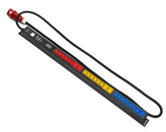
Power strip three-phase SMART PDU, 32A, allows remote monitoring and management of the power distribution system via TCP/IP network. The front panel is equipped with 18 IEC320 C13 outlets and 6 IEC320 C19 outlets. The strip features a color display. Built-in environmental ports enable monitoring of ambient temperature and humidity, door status (open/closed), and the presence of smoke and water through dedicated sensors. It also supports cascading connection of up to 4 additional power strips.
