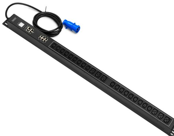
Power strip SMART PDU, single-phase, 16 A, enables remote monitoring and management of the electrical power distribution system via TCP/IP network. The front panel of the strip is equipped with 18 IEC320 C13 outlets and 6 IEC320 C19 outlets. The strip features a color display. Built-in environmental ports allow for monitoring of temperature and humidity levels, door opening, and the presence of smoke or water using dedicated sensors. Cascade connection of up to 4 additional strips is possible.
