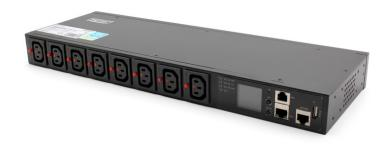
Power strip IPDU H enables switching on/off of outlets and power measurement via TCP/IP. The front panel is equipped with 8 IEC320 C13 outlets. Power ports are individually switchable through a network interface, SNMP, or directly using the button on the control panel. Integration with an additional device (DN-S-BOX) allows the connection of dedicated sensors to monitor: ambient temperature/humidity, door opening/closing, and detect the presence of water or smoke.
