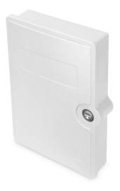
**Outdoor FTTH Box for 6x SC/DX adapter, IP65** FTTH Outdoor Distribution Box IP 65 for 6 SC Duplex Adapter  6 SC Duplex couplers Holder; Splice Protection Holder for 12 Splices; Key lockable; cable overlenght tray; 2 cable entry PG 21; 1 cable entry PG 13.5 mm; fixing material; splice protection, IP 65
