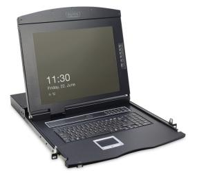
The console can be completely extracted from the server cabinet, and the TFT screen can be tilted through 120 degrees
