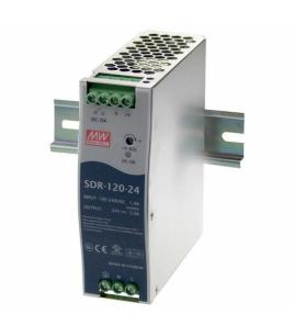
(2.5A), peak 180W (3.75A) for max. 3 seconds. Protection: Short circuit, overload, overvoltage, overheating. Cooling by free air convection, integrated DC OK relay contact, UL 508 (Industrial Control Equipment) and EN61000-6-2 (EN50082-2) compliant, 100% full load burn-in test, Dimensions (WxHxD) 40\*125.2x113.5mm
