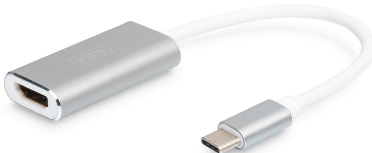
**USB-C 3.2 Gen 1 to HDMI Graphic Adapter 1x HDMI, 4K/30Hz, Aluminium Housing, Silver/White**
