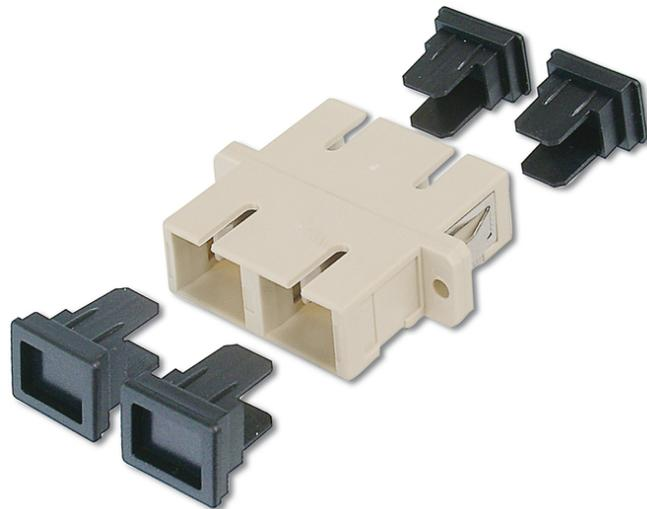
**FO coupler, duplex, SC to SC, MM OM2, color grey ceramic sleeve, polymer housing, incl. screws**
