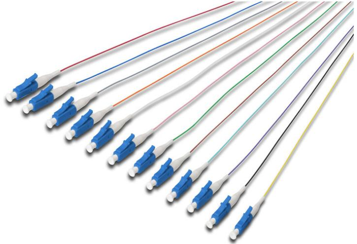
**LWL Pigtail-Set, 12 Stk., LC, SM OS2 09/125 µ loose buffer, Farbcode DIN IEC 304, 2 m**
