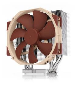
plating Fan compatibility: 140x150x25 (with 120mm mounting holes), 140x140x25 (with 120mm mounting holes), 120x120x25 FAN Specification: Modell: Noctua NF-A15 PWM Bearing: SSO2 Max. Rotational Speed (+/- 10%): 1500 RPM Min. Rotational Speed (PWM, +/-20%): 300 RPM Max. Airflow: 140,2 m³/h Max. Acoustical Noise: 24,6 dB(A) Input Power: 1,56 W Voltage Range: 12 V MTTF > 150.000 h
