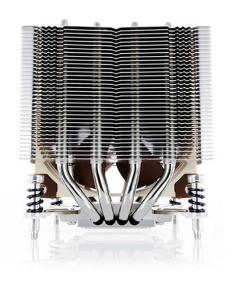
Rotational Speed (PWM, +/-20%): 400 RPM Max. Airflow: 78,9 m³/h Max. Airflow with L.N.A.: 62,6 m³/h Max. Acoustical Noise: 22,8 dB(A) Max. Acoustical Noise with L.N.A.: 16,3 dB(A) Input Power: 1,2 W Voltage Range: 12 V MTBF: > 150.000 h
