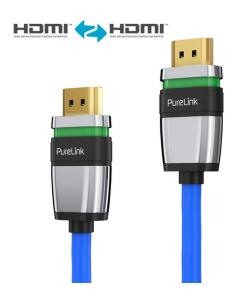
Supported standards High Speed HDMI with Ethernet, ULS Transmission modes Digital audio and video signals Supported Colors 16/24 bit RGB/YUV, Deep Color, x.v.Color™ Supported audio standards ARC, Dolby Digital Plus, Dolby TrueHD, DTS-HD Master Audio™, etc. Maximum resolution 4K / UltraHD / 20160p (4096x2160) @60Hz, 4:4:4
