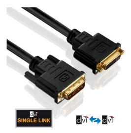
(100% leak) shielding 3 Braid (100% leak) Material outer sheath Highly elastic PVC Outer sheath diameter 7.3mm signal transmission Supported standards DVI Single Link transmission modes Digital video signals Max. Bandwidth 165 MHz Transmission rate max. 3.72 Gbit / s Resolution max. WUXGA (1920x1200) Supported color spaces 8 bit RGB / YUV, Deep Color, xvColor ™ Supported audio standards -More standards HDCP, CEC, full HD (1080i / p), HD ready (720i / p), SDTV (480i / p)
