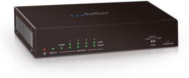
The PT-SP-HD14BT distributes an HDMI input signal via 4x HDBaseT over up to 70 meters for resolutions up to 4K@60 4:2:0. Delivered without HDBaseT receiver. Conections: Input 1x HDMI, 4x IR (3.5mm), 1x IR All-In, 1x RS232 (3-pin Phoenix) Output 4x HDBaseT (RJ45), 1x HDMI (Loop-Out), 1x IR Out, 1x IR Loop-Out, 1x RS232 (3-pin Phoenix)
