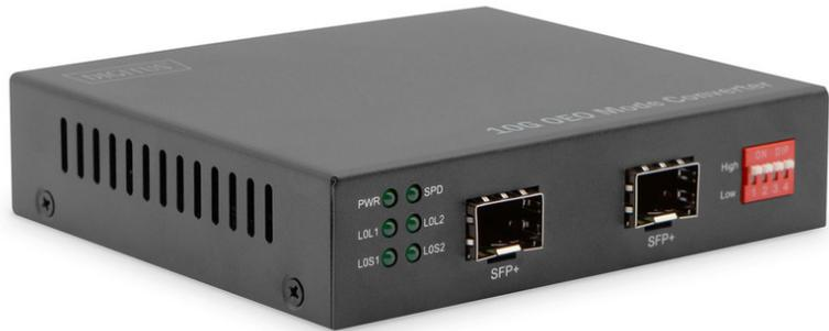
**10G Ethernet Mediakonverter SFP/SFP 1310nm /1550nm/CWDM/DWDM**
