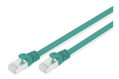
CAT 6A STP flat patch cable, PVC, Cu AWG 30, Length 7.5m , color green
