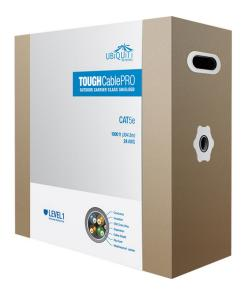
electrostatic discharge (ESD) attacks. Extended Cable Support TOUGHCables have been developed to increase power handling performance for extended cable run lengths. Additional Information: 24 AWG copper conductor pairs 26 AWG integrated ESD drain wire to prevent ESD attacks and damage PE outdoor-rated, weatherproof jacket Multi-layered shielding Available in lengths of 1000 ft (304.8 m)
