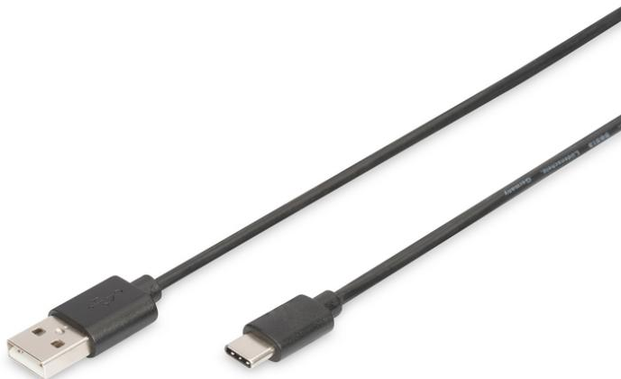
**USB Type-C connection cable, type USB-A to USB-C M/M, 1.8m, 5V3A, 15W, 480Mbps, 2.0 Version, bl**
