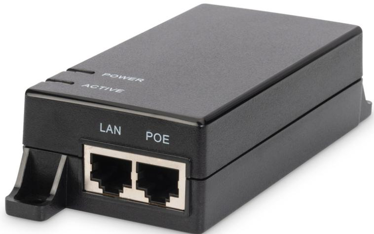
**Gigabit Ethernet PoE Inyector, 802.3af Power Pins:4/5(+),7/8(-), 15.4W**
