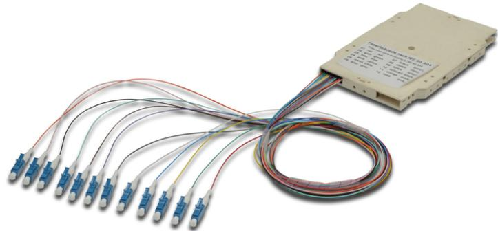
**FO splice cassette with 12 colored pigtails LC (APC), SM OS2 09/125 µm, LSZH**
