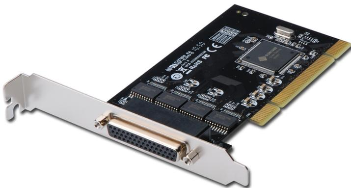
**Serial I/O RS232 PCI Add-On Card 4-port, chipset: SUN1989**
